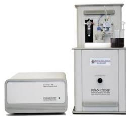
The AccuSizer SIS uses a syringe to deliver an accurate volume of sample through the sensor for analysis. This system is designed for pharmaceutical applications including USP <788> and <787> testing for sub visible particles but provides higher sensitivity and resolution than other available technologies.
