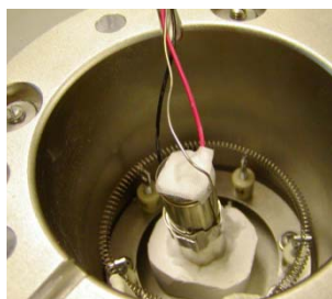
Battery within Calorimeter
