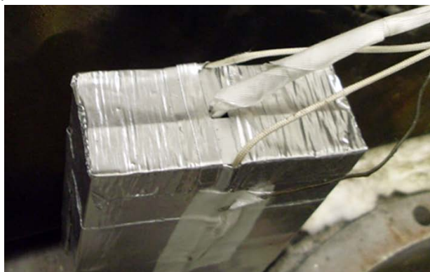
Fig 5 – The aluminium block setup prior to placement in the calorimeter
